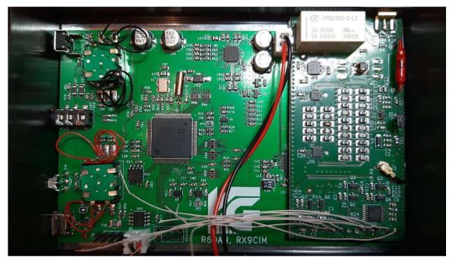
Board power supply can be provided from battery directly or from pcb's power planes. For an example power, can be sourced from capacitor C76 located close to battery connector header, top side is ground ('GND'), bottom is positive ('+').
