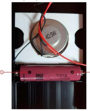
Warning! Observe polarity when inserting battery into battery holder, red wire goes to 'POS' black wire to 'NEG'. Failure to observer polarity would damage radio receiver and void warranty. Check image below for proper installation, check battery polarity with multimeter if polarity is not clear from cell's labels:
